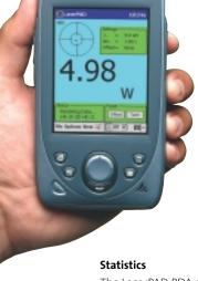
The LaserPAD PDA can perform complete statistical and power trend analysis for stability and drift measurements. From 40 to 2000 data points can be recorded and analyzed over a selected period of time for display on a strip chart or histogram plot.
